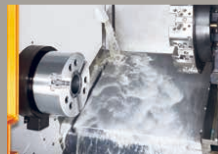
Coolant flush onto covers (Photo with opt. pump Grundfos MTH4-40/4)
